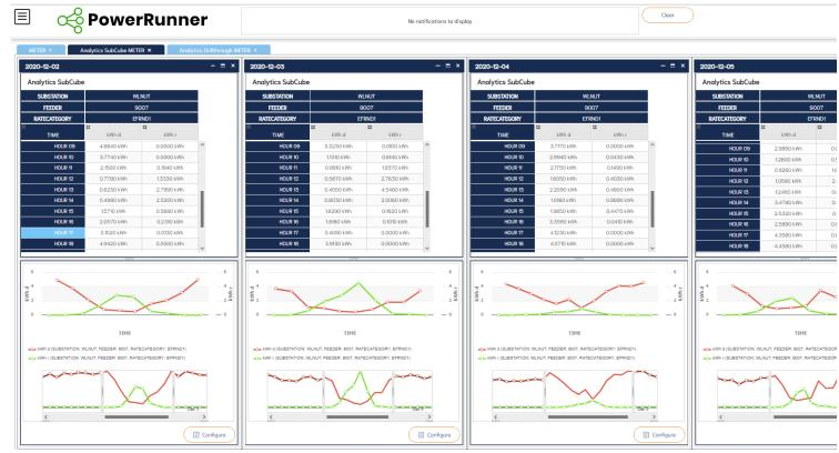
Substation, Feeder, rate category, hour, energy delivered, energy received
